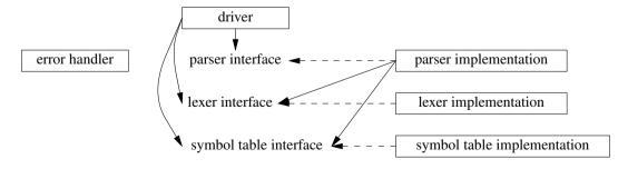
A dashed line means "implements." I consider this to be the real structure of the program, and our job as programmers is to represent this faithfully in code. That done, the code will be simple, efficient, comprehensible, maintainable, etc., because it will directly reflect our fundamental design.
