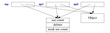
The "weak use count" is needed to keep the use count structure alive because there may be weak ptrs after the last shared ptr for an object (and the object) is destroyed.
