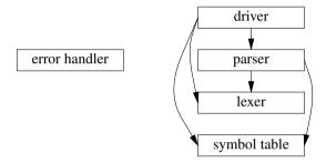
where an arrow means "using." To simplify the picture, I have not represented the fact that every part relies on error handling. In fact, the calculator was conceived as three parts, with the driver and error handler added for completeness.
